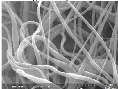
Figure 3 – SEM image of the inside of the condensed nanofibrous bundle
