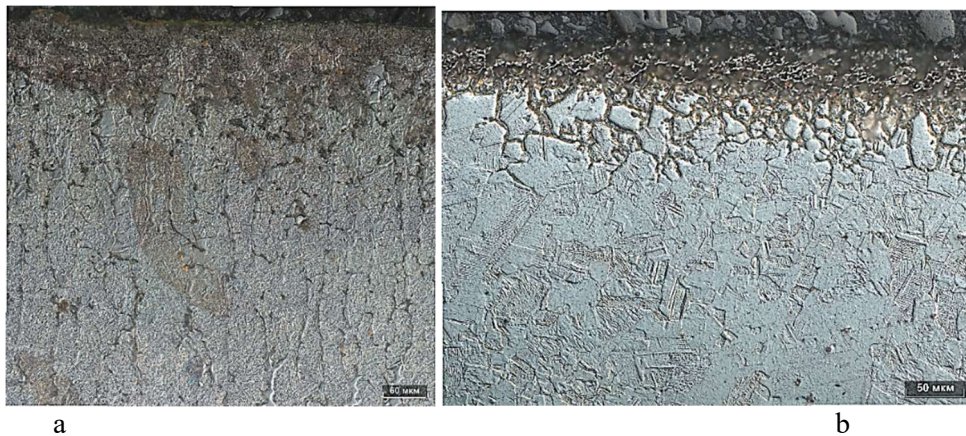
Figure 1 – The microstructure of the diffusion coating, obtained by simultaneous saturation of boron and carbon on steels: a – AISI 430, b – AISI 303
